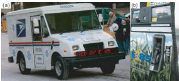
Figure 5.33: Ethanol provides up to 85% of the energy needs of new “fuel-flex” cars. Although its energy efficiency is still controversial, ethanol from corn or cellulose appears to be more “renewable” than fossil fuels.
