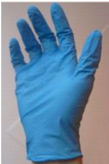
Figure 1.48: A nitrile glove. Latex gloves are no longer recommended so vinyl gloves or nitrile gloves, which are usually green or blue in color, are preferred.
