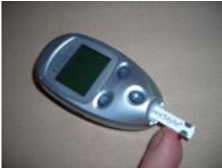
Figure 19.8: A person with diabetes has to monitor their blood glucose carefully. This glucose meter analyses only a small drop of blood. For an animation of diabetes, see (
