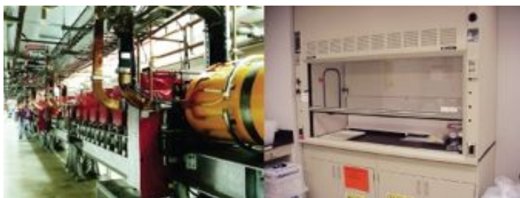
Figure 1.35: Different fields of science need different types of equipment, such as the particle accelerator at left, found in a physics lab, and the fume hood, at right, found in chemistry labs, but also sometimes in biology labs.
