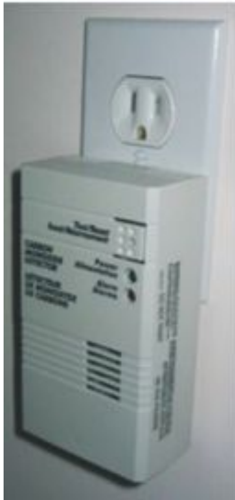
Figure 24.24: Home carbon monoxide detector
