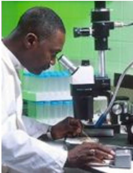
Figure 1.38: This scientist is using a stereo microscope, which is a light microscope with two ocular lenses (the microscope lens that is closest to the eye). The microscope is fitted with a digital imaging device that can take digital photos of what the researcher sees.
